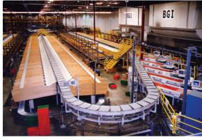
A typical Mantissa solution consists of a combination of fast conveyer belts, trays and discharge chutes. As product is transported through a facility it all arrives at the Mantissa sorter trays, which are arranged in a train-like fashion and operate along a track. Then patented control systems automatically sort and distribute material into chutes for further processing. Basically, the equipment looks like an 800-foot racetrack inside a commercial building.
